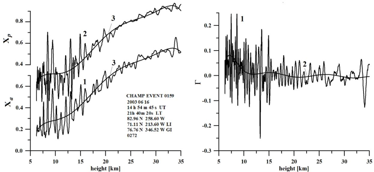
**Figure 3.** Left. Comparison of the refractive attenuation  $X(h)$  retrieved from the eikonal data and attenuation  $X_a(h)$  found from the intensity variations of the RO signal. Right. Difference of the refractive attenuations  $X - X_a$  (curve 1) and absorption coefficient  $\Gamma$  found by a least-squares method (curve 2).
