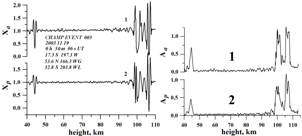
**Figure 5.** Left plot: the refractive attenuations  $X_a, X_p$  found from the intensity and eikonal ro data at frequency  $f_1$  (curves 1 and 2, respectively). Right plot: the amplitudes  $A_a, A_p$  of analytical signals corresponding to the variations of the refractive attenuations  $X_a, X_p$  (curves 1 and 2).
