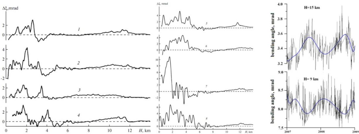
**Figure 8.** Left panel. Examples of the refractive angle variations obtained in January 2007. Middle panel. Examples of the refractive angle variations obtained in July 2010. Right panel. Annual changes of the bending angle at the 9 km and 15 km altitudes from FORMOSAT-3 RO data in Moscow region.
