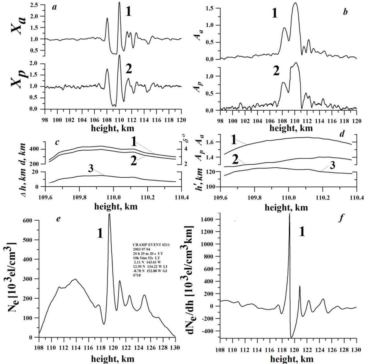
**Figure 7.** Panels a-d: identification and location of a layer in the lower ionosphere. Panel e: distribution of the electron density in the identified sporadic Es layer. Panel f: distribution of the gradient of electron density.
