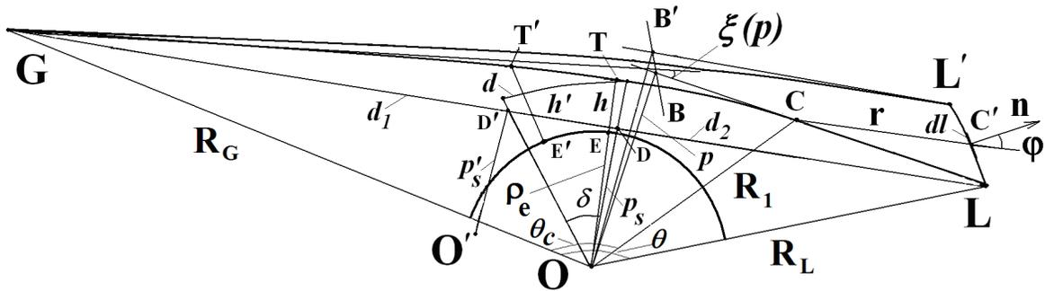
**Figure 2.** Main geometrical parameters describing the RO experiment conditions.
