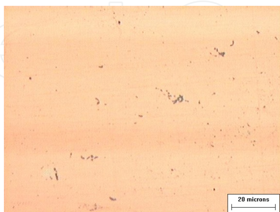
Figure 17. Optical micrograph of the ternary alloy Cu-1.0%Ni-0.5%Cr, cold compact (20MPa) and sintered at 1073K for 5.4 \times 10^3 s and homogenized at 773K for 172.8 \times 10^3 s.
