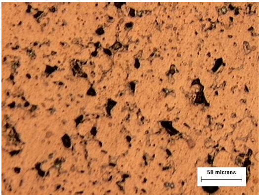
Figure 11. Optical micrograph of the ternary alloy Cu-0.5%Ni-0.5%Cr, cold compact (20MPa) and sintered at 1053K for 5.4x10 3 s and also homogenized at 773K for 32.4x10 3 s.
