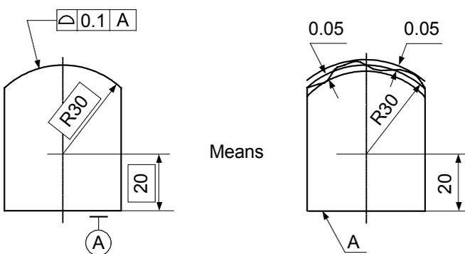
Figure 1. Interpretation of profile of a relevant surface
