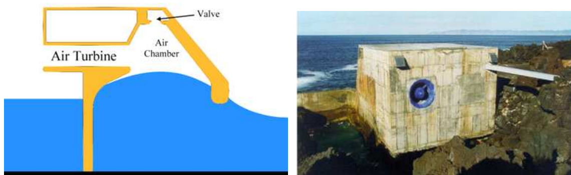
Figure 20. Left side: Schematic of OWC. Right side: Back view of an OWC [37].
