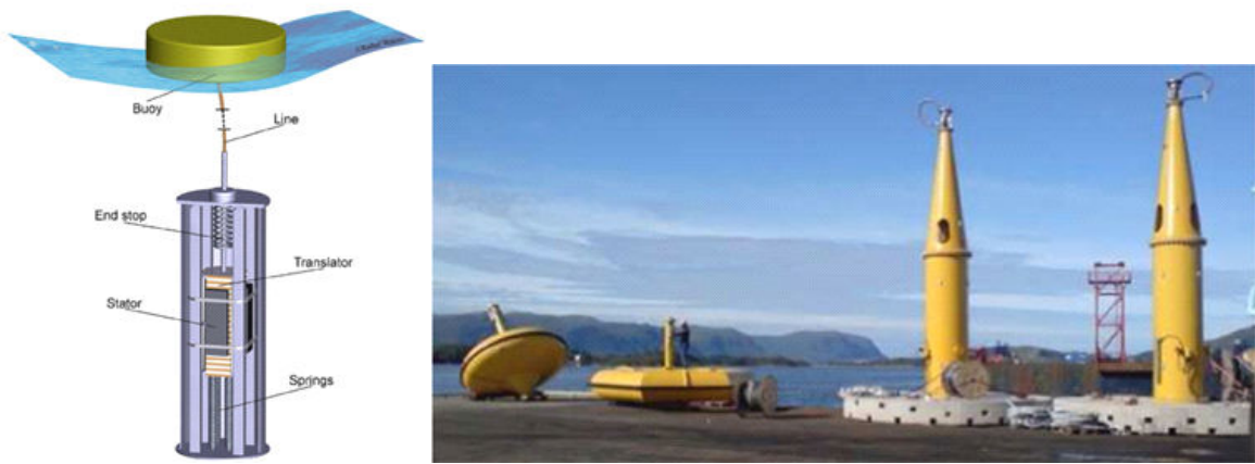
Figure 8. Left side; Taut moored heaving buoy with linear electrical machine PTO [16]. Right side; Component of taut moored WEC, Sweden [22].
