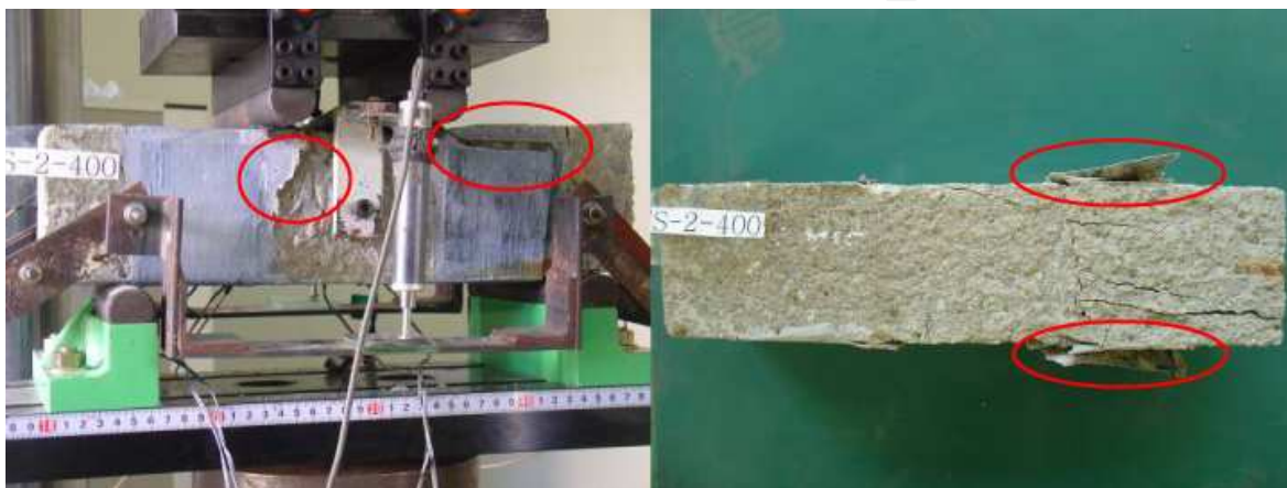
Figure 3. De-lamination of CFRP at failure
