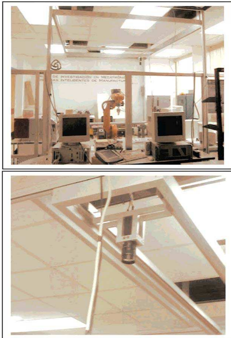
Figure 7. Vision workspace. Overview and 2D close up of positioning system
