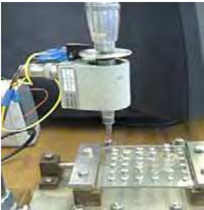
Figure 8. A screwdriver attached transducer and encoder
