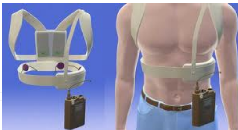
Figure 7. LifeVest®, ZOLL: main components and how it should be worn.
