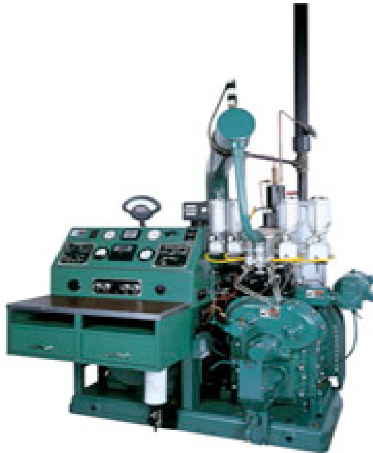
Figure 2. CFR engine for MON octane (WAUKESHA, 2012)
