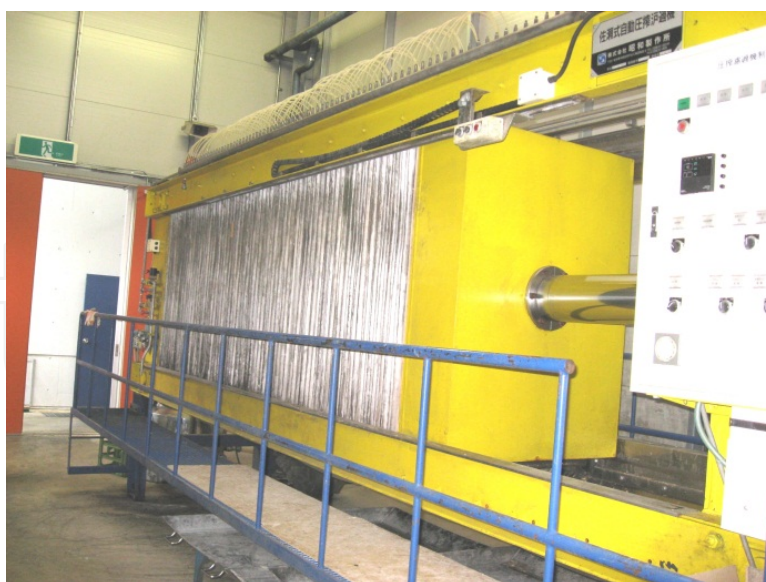
Figure 8. SAKE squeezer (Photograph by Hamada Co. Ltd)
