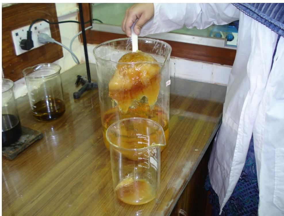
**Figure 6.** Separation of glycerin from Biodiesel
