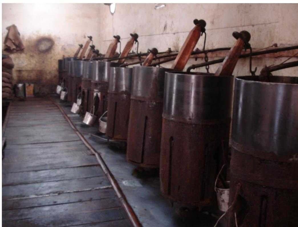
**Figure 3.** Mechanical Oil Expeller
