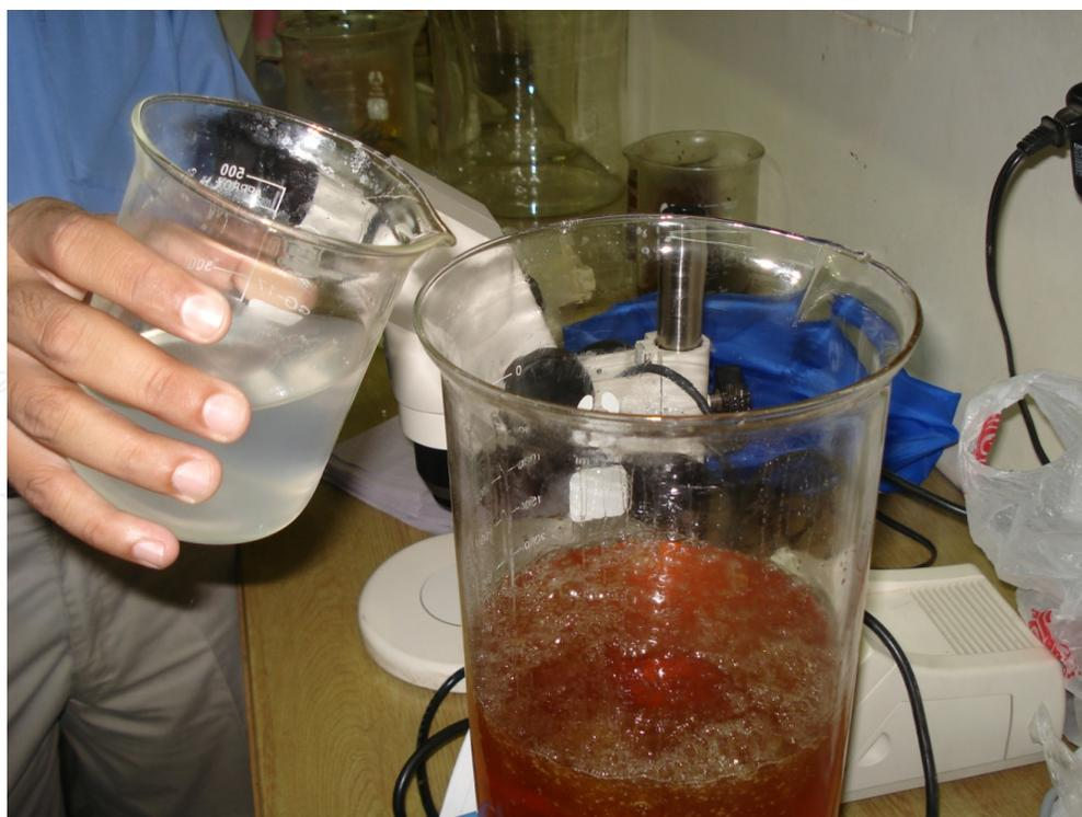
**Figure 5.** Mixing of catalyst
