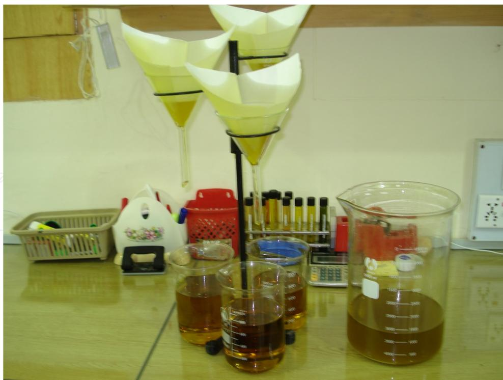
**Figure 7.** Biodiesel Filtration
