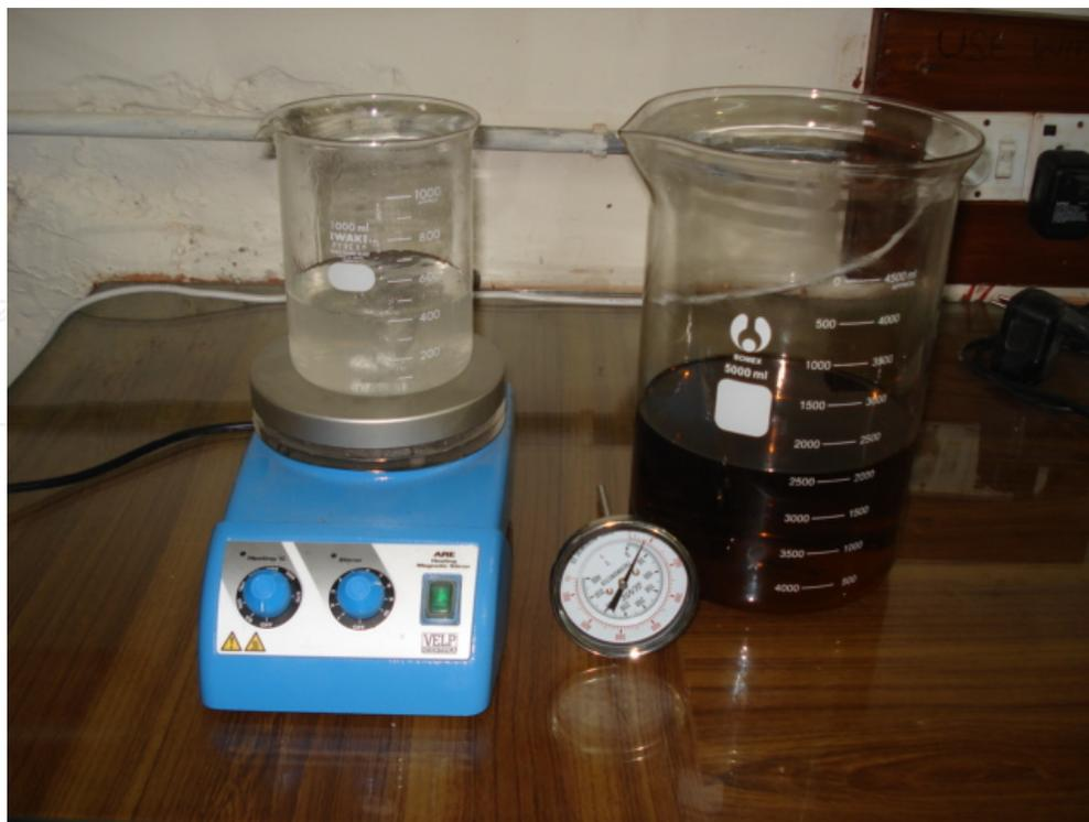
**Figure 4.** Preparation of Methoxide catalyst
