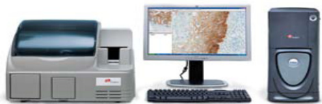
Figure 1. Automated Cellular Imaging System (ACISR III), an example of an image acquisition and image analysis instrument.
