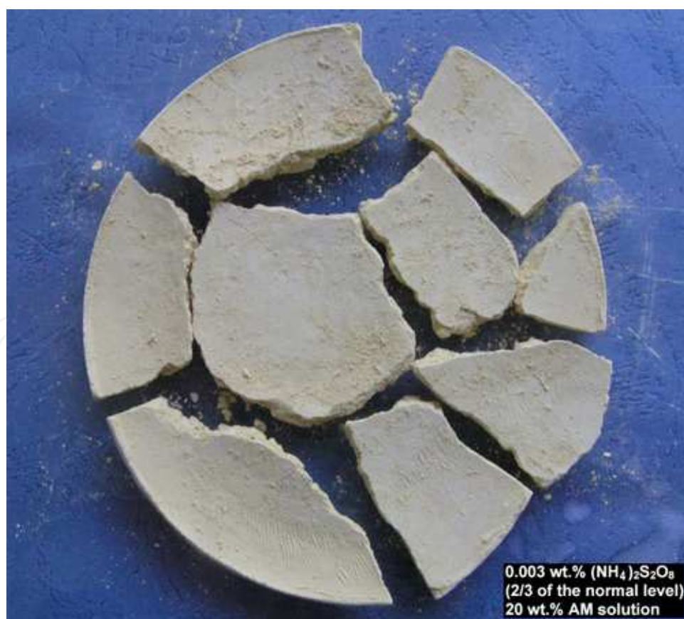
Figure 11. A fractured PZT-4 type green body caused by a lower initiator concentration
