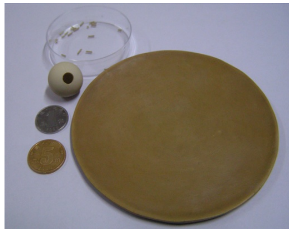
Figure 13. Illustration of special-shaped gelcast PZT ceramics: spherical PZT plate and hollow spherical PZT shell.
