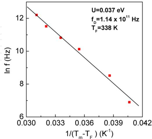
**Figure 6.** Temperature dependence of the frequency ( $\ln f$  versus  $1/(T_m - T_F)$  curve) for PLZT 10/80/20 ferroelectric ceramic system. Solid lines represent the fitting by using the Vogel–Fulcher relation.
