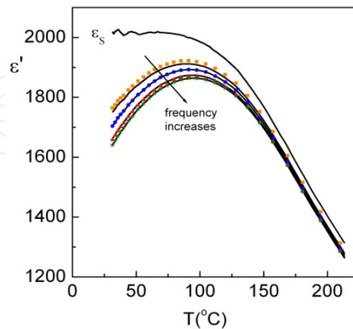
**Figure 3.** Temperature dependence of the real part ( $\varepsilon'$ ) of the dielectric permittivity at several frequencies for PLZT 10/80/20 ferroelectric ceramic system. The experimental values are represented by solid points and the theoretical results by solid lines. It has been included the theoretical temperature dependence of the static dielectric permittivity ( $\varepsilon_s$ ).
