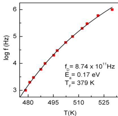
**Figure 14.** Dependence of the  $\log f$  with  $T_m$  for the  $\text{Sr}_{0.5}\text{Ba}_{0.5}\text{Bi}_2\text{Nb}_2\text{O}_9$  considering a frequency range from 1 kHz to 1 MHz. The fitting was carried out by using the Vogel-Fulcher law.
