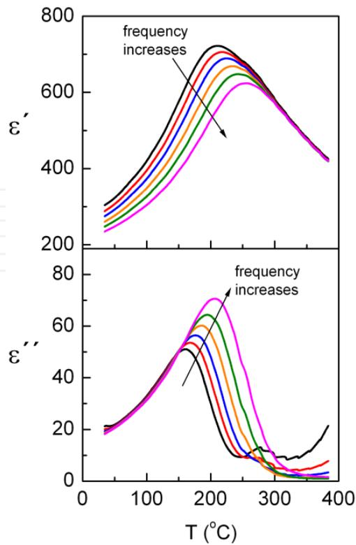
**Figure 12.** Temperature dependence of the real ( $\epsilon'$ ) and imaginary ( $\epsilon''$ ) parts of the dielectric permittivity, at several frequencies, for the  $\text{Sr}_{0.5}\text{Ba}_{0.5}\text{Bi}_2\text{Nb}_2\text{O}_9$ .
