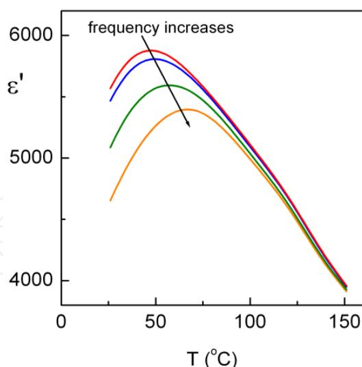
**Figure 10.** Temperature dependence of the real ( $\epsilon'$ ) part of the dielectric permittivity at several frequencies for  $(\text{Pb}_{0.8}\text{Ba}_{0.2})[(\text{Zn}_{1/3}\text{Nb}_{2/3})_{0.7}\text{Ti}_{0.3}]\text{O}_3$  ferroelectric ceramic system.
