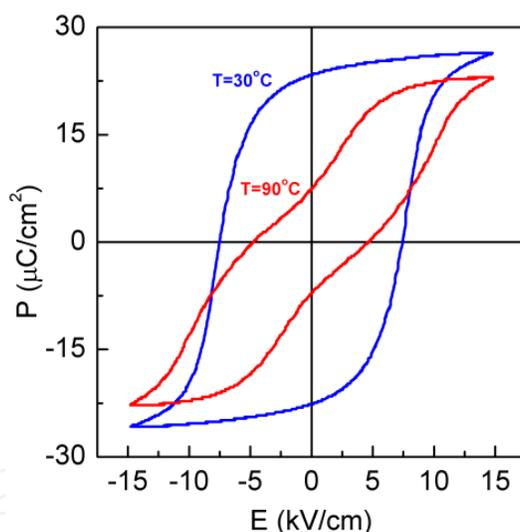
**Figure 2.** Hysteresis loops for PLZT 6/80/20 ferroelectric ceramic system.
