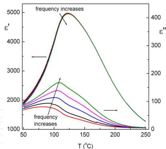
**Figure 1.** Temperature dependence of the real ( $\epsilon'$ ) and imaginary ( $\epsilon''$ ) parts of the dielectric permittivity at several frequencies for PLZT 6/80/20 ferroelectric ceramic system.
