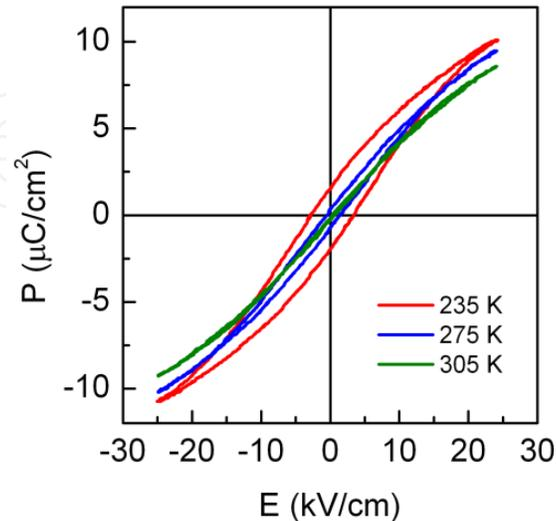
**Figure 11.** Hysteresis loops for  $(\text{Pb}_{0.8}\text{Ba}_{0.2})(\text{Zn}_{1/3}\text{Nb}_{2/3})_{0.7}\text{Ti}_{0.3}\text{O}_3$  ferroelectric ceramic system.
