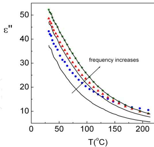
**Figure 4.** Temperature dependence of the imaginary part ( $\epsilon''$ ) of the dielectric permittivity at several frequencies for PLZT 10/80/20 ferroelectric ceramic system. The experimental values are represented by solid points and the theoretical results by solid lines.
