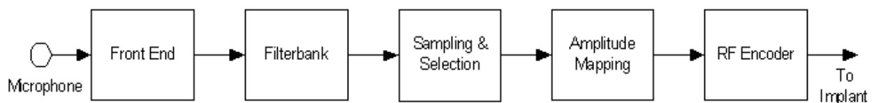
Figure 3. Audio signal path used in current filterbank strategies (Swanson, 2007).
