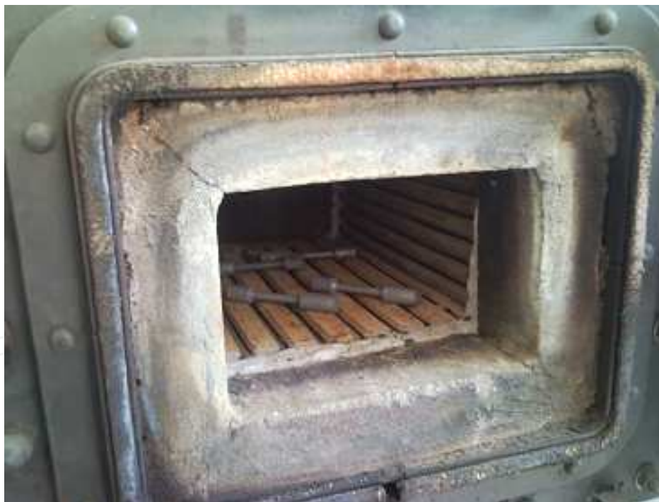
Figure 2. The Photograph of the furnace that is used for homogenization treatment.
