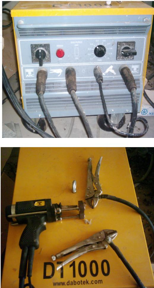
**Figure 4.** The DABOTEK stud welding machine
