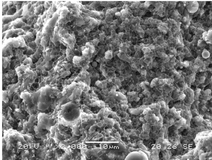
Figure 4. Fractograph of the laser welded joint with 0.3 mm thick Ti filler
