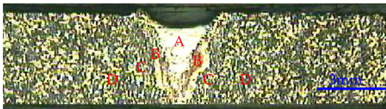
Figure 6. Macro-structure of the laser welded joint with 0.3 mm thick Ti filler
