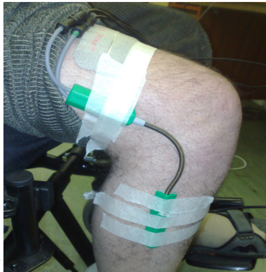
Figure 3. Electro-goniometer arrangement for pendulum test
