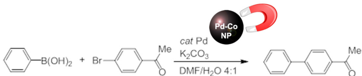
Figure 23. Suzuki reaction by using Pd or Pd@Co nanocomposites with optimized conditions.
