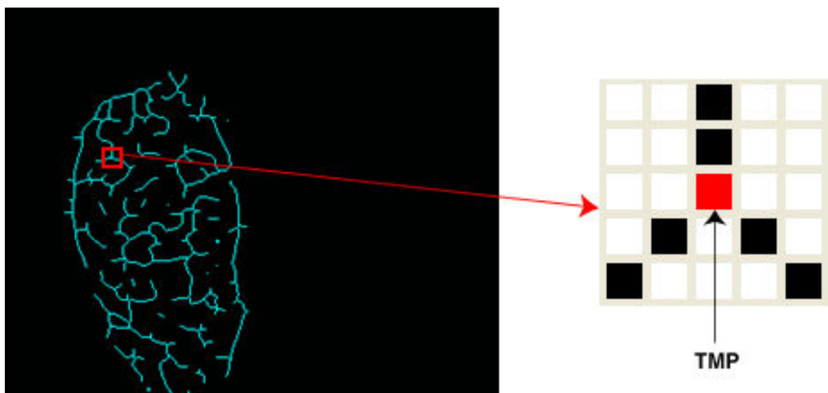
Figure 18. A thermal minutia point being extracted from a thinned vascular network[29].
