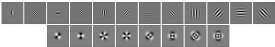
Figure 19. The Gabor (first row) and Laguerre-Gaussian (second row) filter banks.
