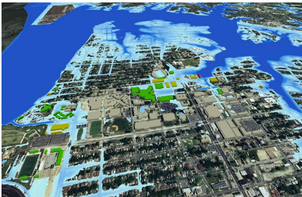
Figure 11. A 3-D ortho-perspective of Hurricane Irene maximum flooding at ODU campus. Map depicts inundation depth superimposed over 3-D buildings and orthophotography draped on a LiDAR DEM. View north toward Lafayette River at top and Elizabeth River at left. Inundated areas shown in blue shades connote inundation depths (as described in Figure 5). Building hues denote water level at first floor base height of building.
