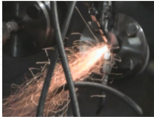
Figure 14. Picture showing the syngas flame caused by syngas leakage at the feed nozzle area
