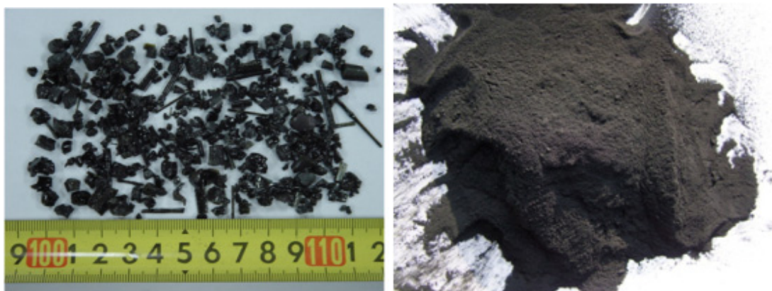
Figure 4. Slag(left) from slagging gasifier and fly-ash(right) from non-slagging gasifier
