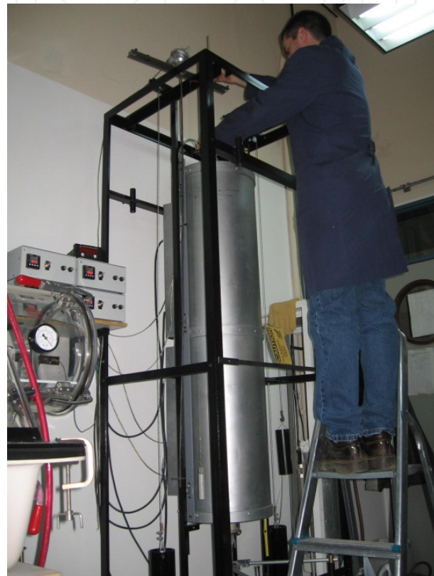
Figure 1. Drop tube furnace for pyrolysis experiments: (a) schematic view; (b) photograph taken during assembly.
