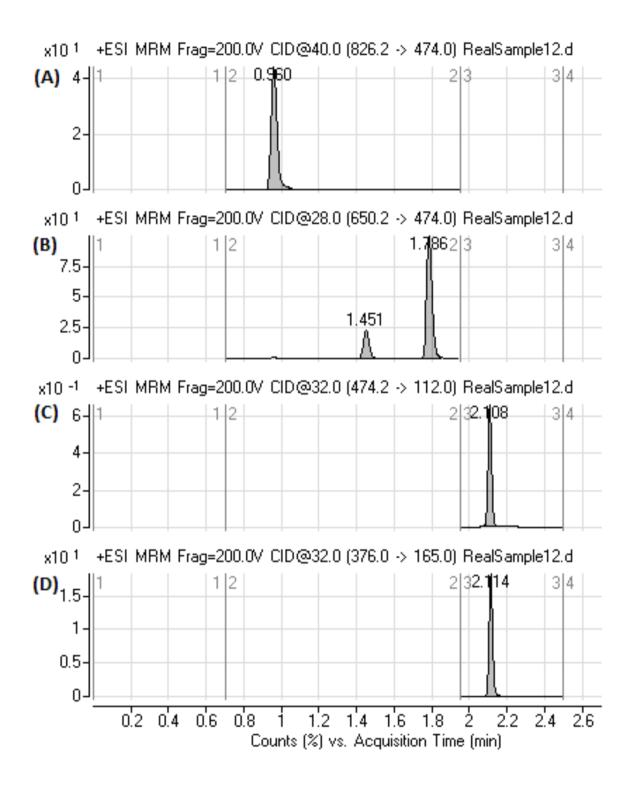
**Figure 1.** LC-MS/MS chromatogram of urine sample from a patient receiving raloxifene. MRM transitions represent (A) raloxifene diglucuronide, (B) two raloxifene monoglucuronides (C) parent raloxifene, (D) haloperidol as internal standard. For analysis conditions refer to [37].
