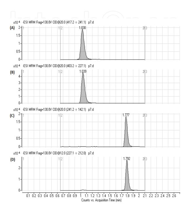
**Figure 2.** LC-MS/MS chromatogram in MRM mode for metabolite (BPAG) and parent bisphenol A (BPA) of a typical microsomal incubation. (A) mass transition for BPAG<sub>d16</sub> (internal standard for BPAG), (B) mass transition for BPAG, (C) mass transition for BPAd<sub>16</sub> (internal standard for BPA), (D) mass transition for BPA. For analysis conditions refer to [4].
