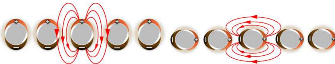
Figure 7. Schematic of near-field coupling between metallic NPs for two different polarizations.
