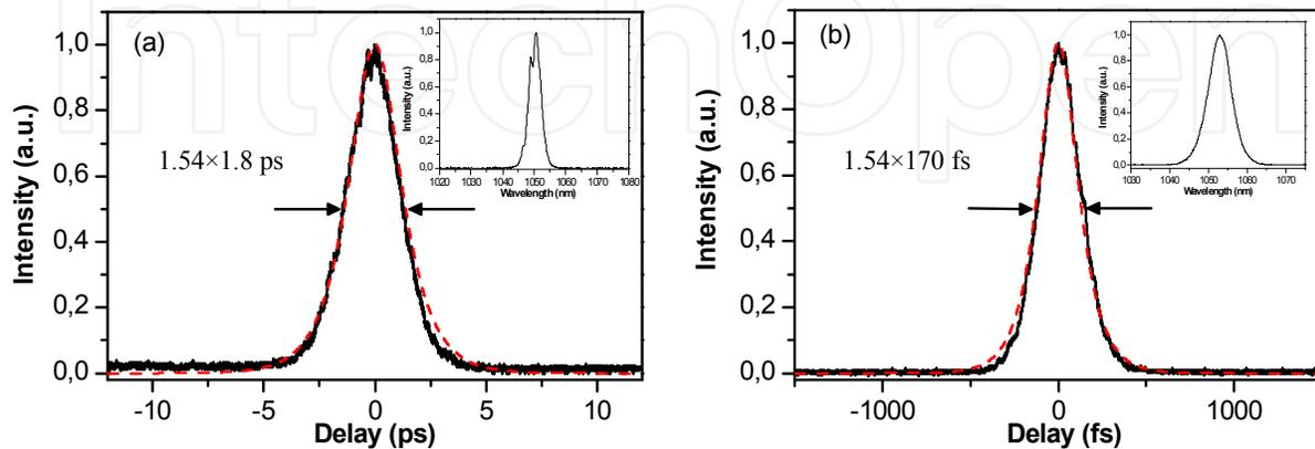
**Figure 16.** (a) Intensity autocorrelation trace of the picosecond pulses; inset, the corresponding laser spectrum. (b) Intensity autocorrelation trace of the femtosecond pulses; inset, the corresponding laser spectrum.
