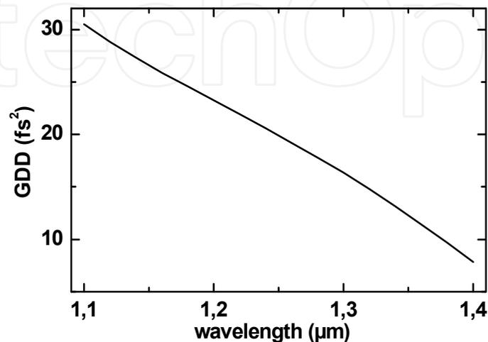
**Figure 27.** Group-delay dispersion from 1 mm Cr<sup>4+</sup>:forsterite crystal
