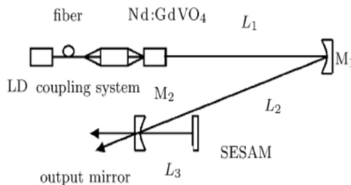
**Figure 9.** Schematic diagram of the passively mode-locked 912 nm Nd:GdVO<sub>4</sub> laser.
