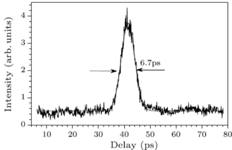
**Figure 12.** Autocorrelation trace of the mode-locked Nd:LuVO<sub>4</sub> laser.
