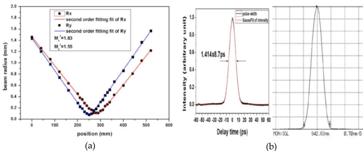
**Figure 4.** (a) Measured  $M^2$  for tangential direction (Rx) and sagittal direction (Ry); (b) left: Intensity autocorrelation trace of the pulse; right: The laser spectrum of mode-locking operation.
