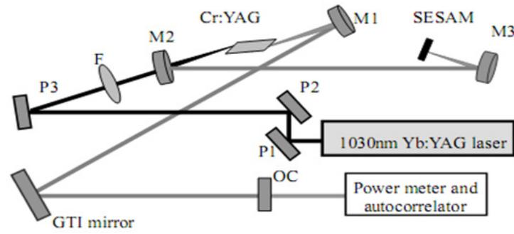
**Figure 31.** The schematic diagram of the self-starting mode locking Cr<sup>4+</sup>:YAG laser.
