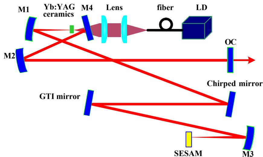
**Figure 17.** Schematic of the mode-locked Yb:YAG ceramic laser.
