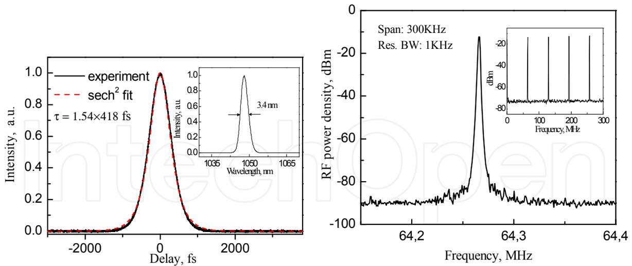
**Figure 19.** Left, intensity autocorrelation trace of the mode-locking laser pulses with 1.9 W average power; inset, the corresponding spectrum. Right, the rf spectrum at fundamental repetition frequency of the 418 fs pulse train; inset, resolution bandwidth of 100 kHz and span of 300 MHz.
