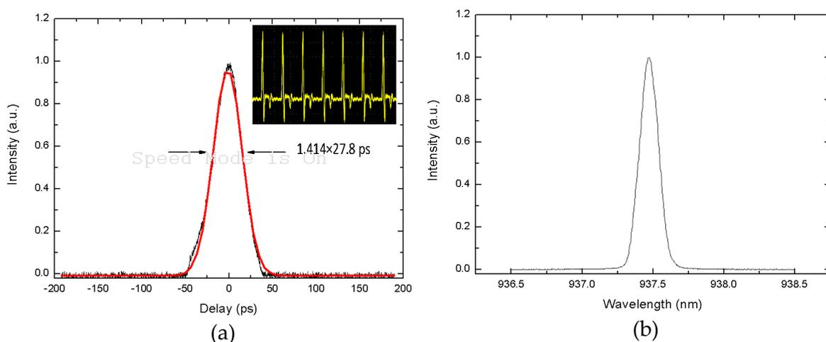
**Figure 8.** (a) Intensity autocorrelation together with Gaussian fit curve shows the pulse width of 24.7 ps. The inset is oscilloscope traces of the CW mode-locked pulse train. The laser spectrum of mode-locking operation.
