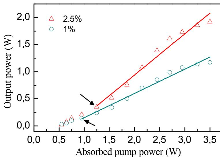
**Figure 18.** Average output power versus absorbed pump power of the mode-locked Yb:YAG ceramic laser with output couplings of 2.5% (triangles) and 1% (circles). The cw mode-locking thresholds are indicated by arrows.
