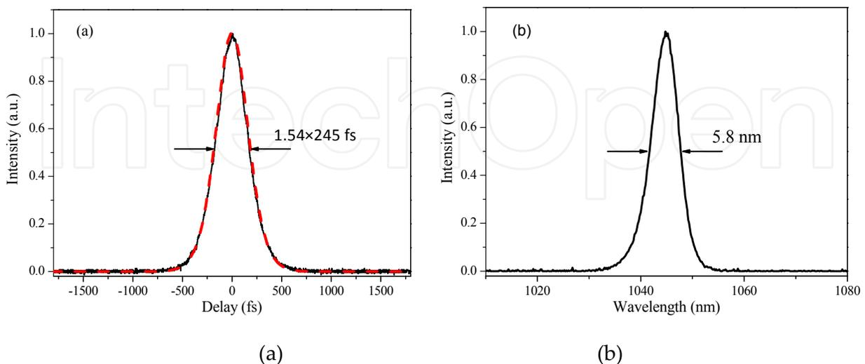
**Figure 24.** (a) Intensity autocorrelation trace of the pulse. The experimental data are shown by the solid curve and the  $\text{sech}^2$ -fitting curve by the dashed curve. (b) The laser spectrum of mode-locking operation.
