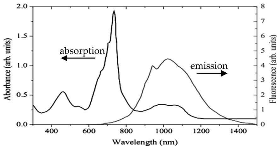
**Figure 25.** Absorption and emission spectrum of Cr<sup>4+</sup>:forsterite
