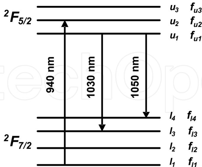
**Figure 13.** Energy level diagram of Yb<sup>3+</sup> ion in the Yb:YAG crystal.
