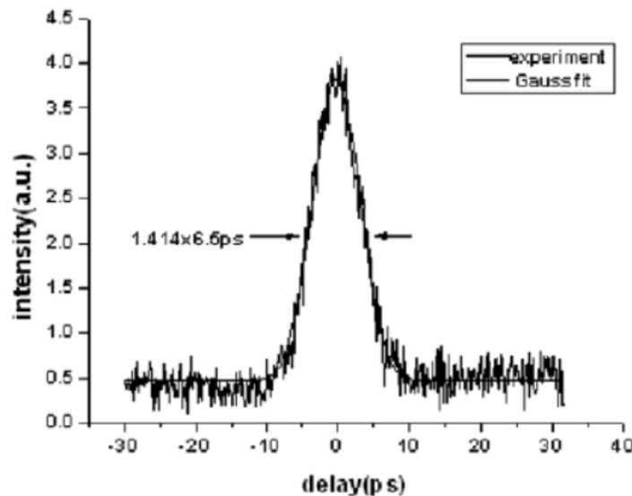
**Figure 11.** The measured autocorrelation trace of the pulses of the passively mode-locked 912 nm Nd:GdVO<sub>4</sub> laser.
