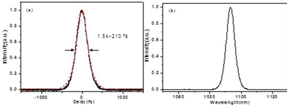
**Figure 22.** (a) Typical intensity autocorrelation trace of the pulses. The experimental data are shown by the solid curve and the sech<sup>2</sup>-fitting curve by the dashed curve. (b) The laser spectrum of mode-locking operation.
