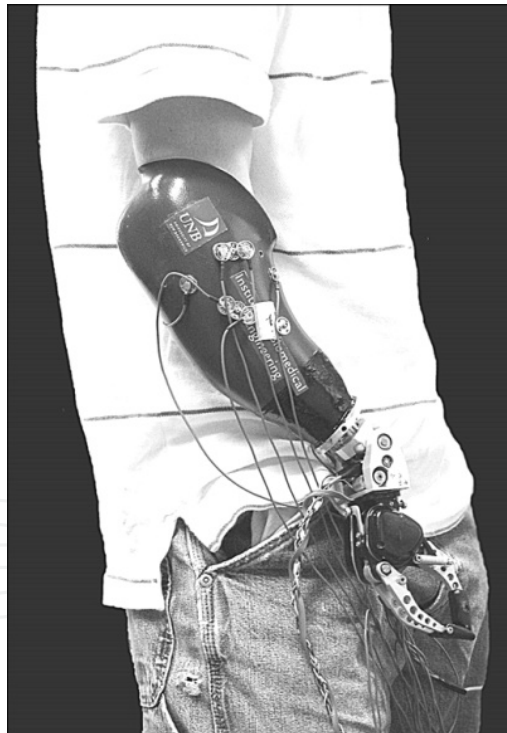
Figure 1. An experimental setup for a myoelectric prosthesis, developed at the University of New Brunswick, Canada (extracted from [18]).
