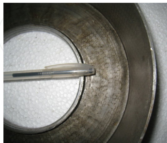
b) Part with inner wall thickened by upsetting
