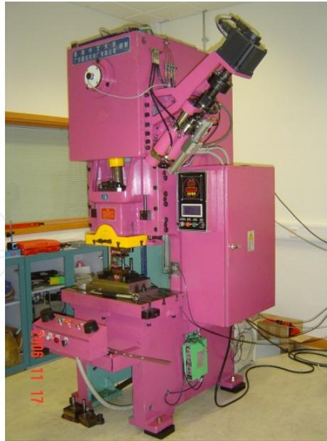
**Figure 2.** The prototype of a hybrid press
