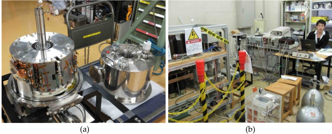
Figure 14. (a) A prototype bulk HTS motor designed for a specification of 30 kW 720 rpm and (b) a homemade pulsed-field magnetization system (TUMSAT-OLCR). This is an axial-type machine with a thermosyphon cooling system using Ne.
