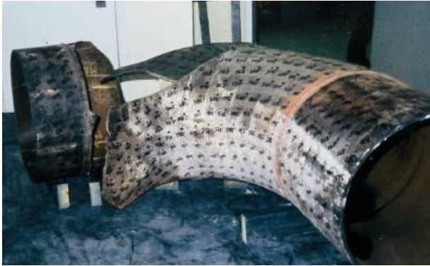
18" elbow wall thickness decreased from 12.7 to 1.5 mm on feed-water pump inlet at Surry, 1986
