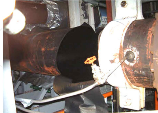
Wall Thickness reduced from 10 to 1.5 mm on Feed-water piping at Mihama unit 3, 2004
