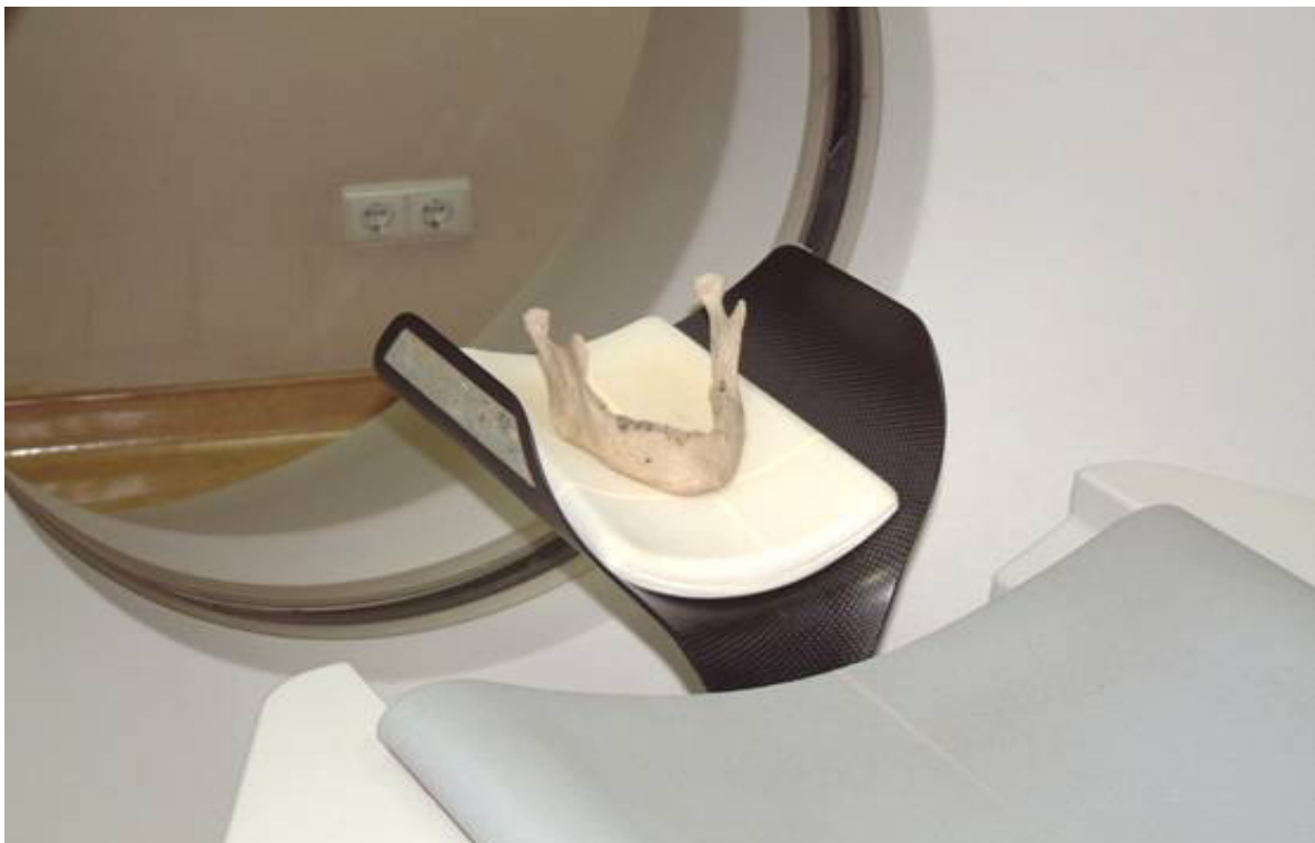
Figure 16. The edentulous mandible obtained from a cadaver was scanned using a dental volumetric tomography device
