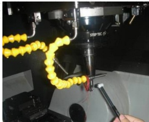
Figure 15. Experiment setup for modal shapes of spindle-tool system
