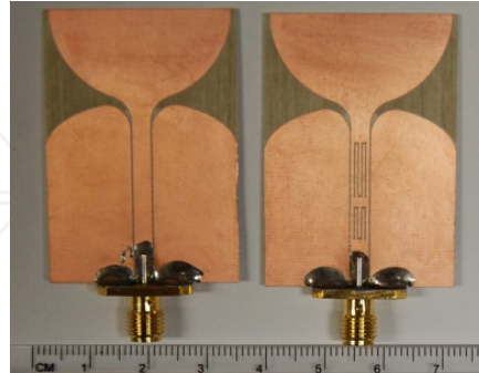
Figure 7. Photograph of CPW antennas without and with dual-band CPW resonator
