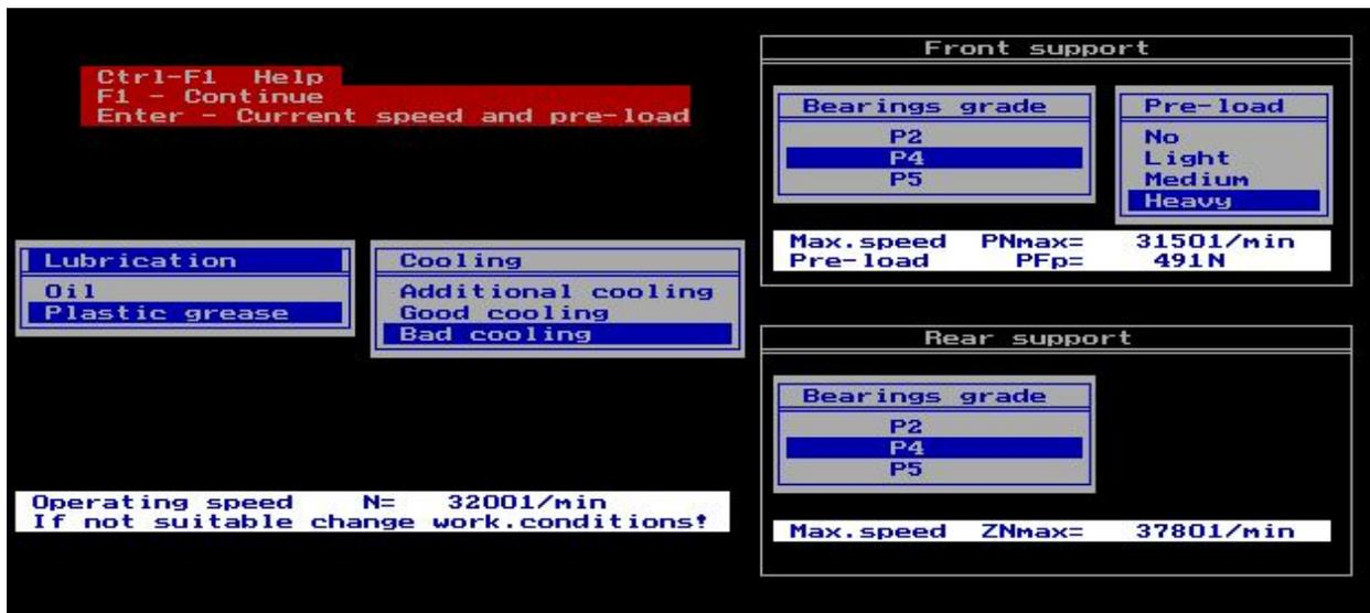
**Figure 20.** Entering preliminary data for the bearings conditions
