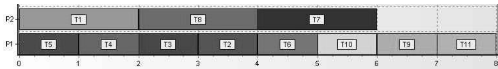
Figure 27. Optimal scheduling for the problem solved with Baer algorithm, obtained as a result of ACO algorithm use
