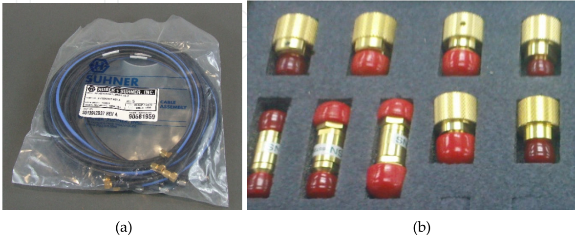
Figure 10. (a) coaxial cables (b) Agilent 85052 D calibration kit
