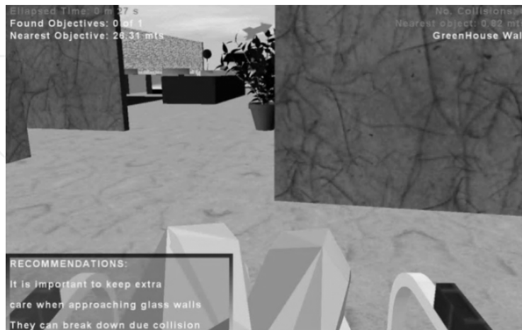
Figure 29. This image shows the virtual trainer along with the augmented reality interface. In the upper left corner, information about the performance of the user is shown: elapsed time, found targets. In the upper right corner there are more statistics such as number of collisions and the name of the nearest object. In the lower area data that can help the user to navigate more properly or about the closest
