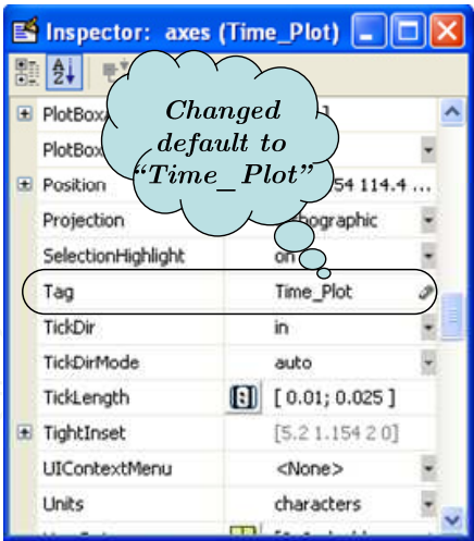
Figure 3. The property inspector of Axes1 assigned name to "Time_Plot".
