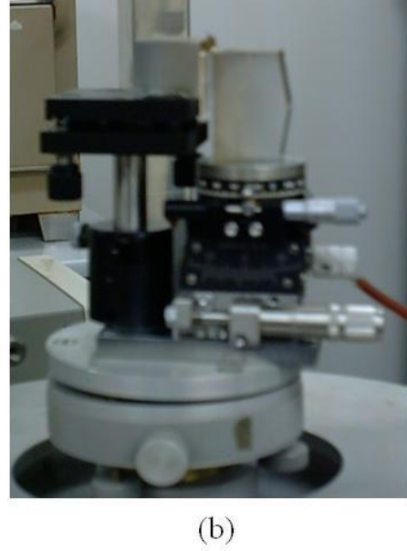
Figure 15. Displacement sensor of intensity interrogation (a) structural sketch; (b) actual picture
