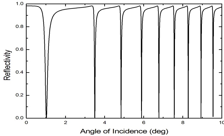
Figure 3. Simulated ATR curve with the following parameters: \varepsilon_2 = -28 + i1.8 , \varepsilon_1 = 2.278 , \lambda = 859.8 \text{ nm} , h = 30 \text{ nm} , and d = 0.38 \text{ mm} .
