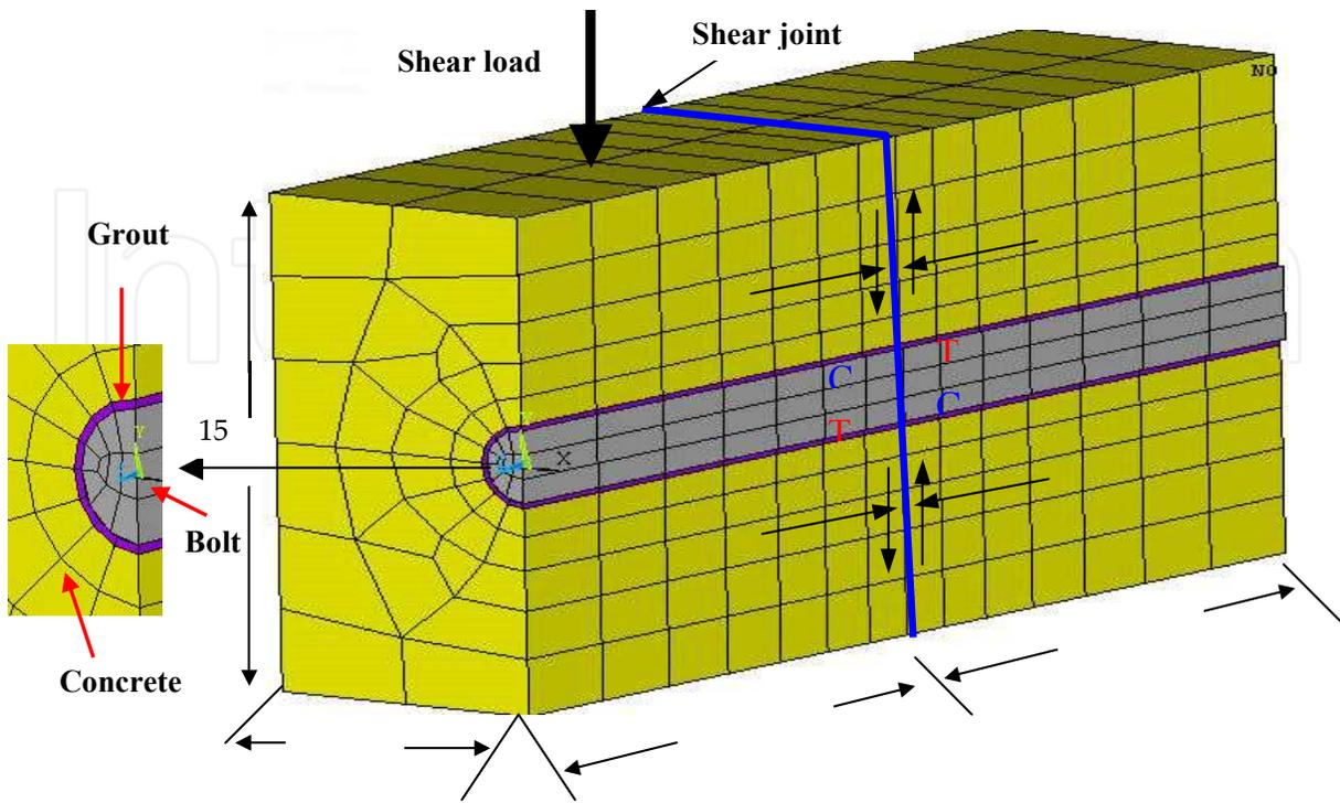
Figure 9. Geometry of the model and mesh generation
