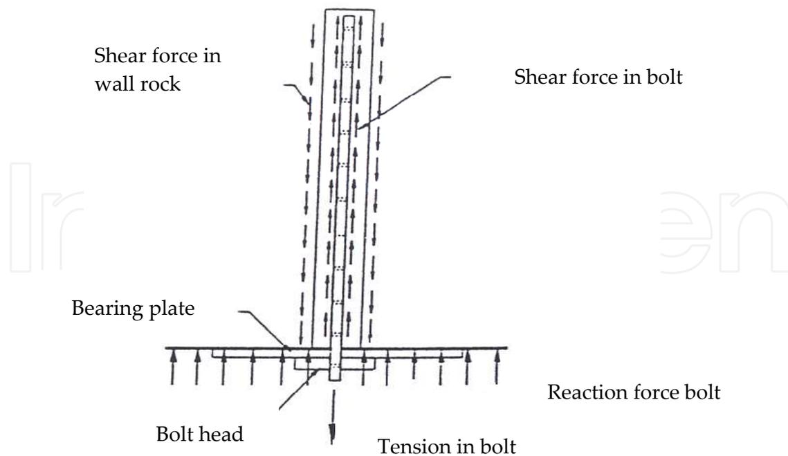
**Figure 3.** Bolt-Rock interaction model (after Peng and Guo, 1992)
