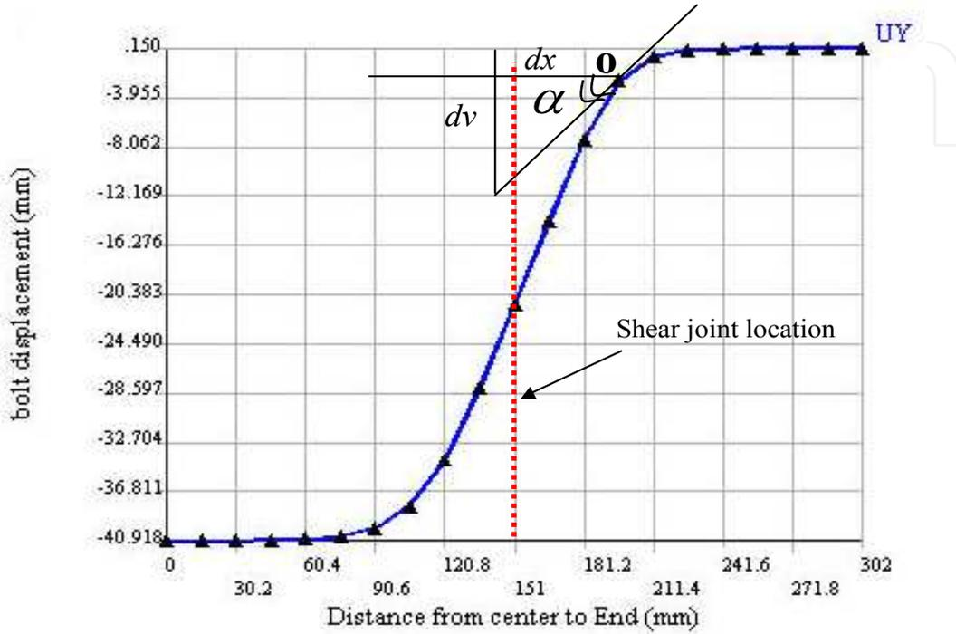
Figure 12. Bolt displacement in 20 MPa, without Pre-tension
