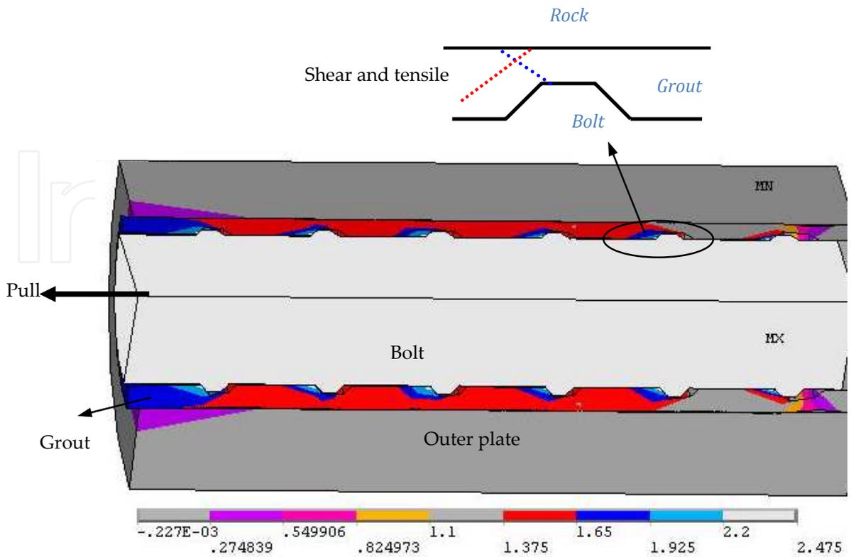
**Figure 37.** The bolt movement in pulling test
