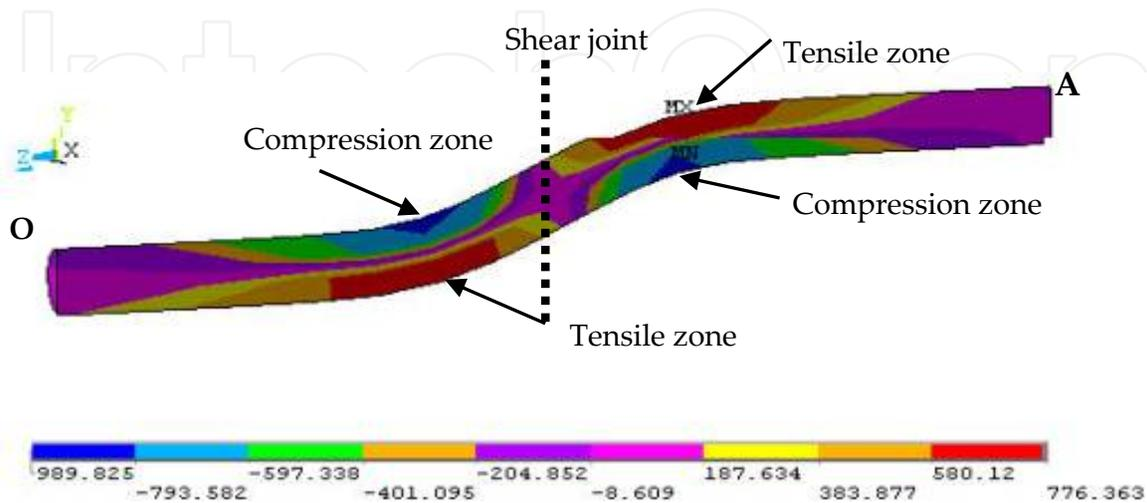
**Figure 15.** Stress built up along the bolt axis in 20 MPa concrete without pre-tension
