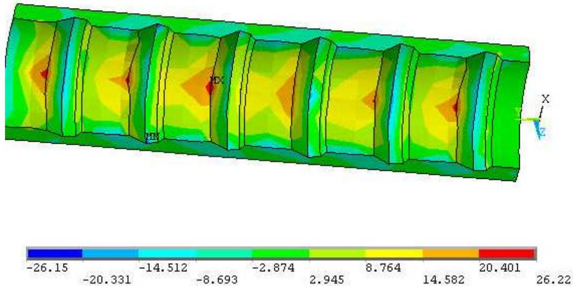
**Figure 40.** Shear stress contours along the grout interface
