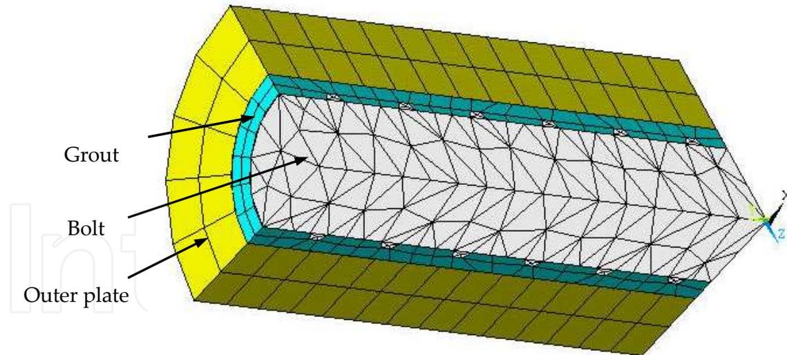
**Figure 36.** FE mesh: a quarter of the model
