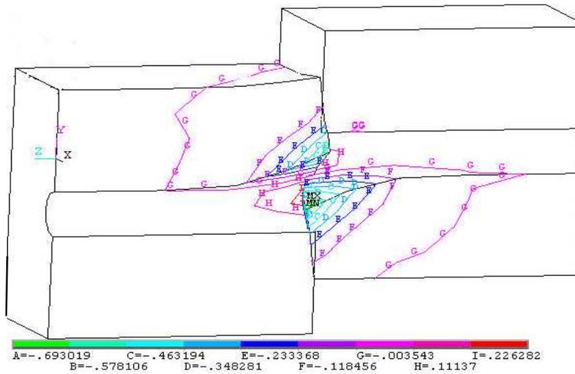
Figure 29. Strain contours in 20 MPa concrete without pre-tension
