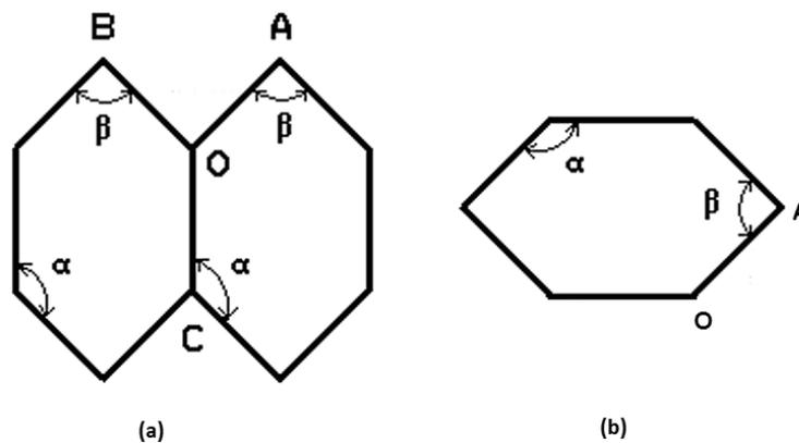
**Figure 3.** a) Two units of a zigzag CNT. (b) One unit of an armchair CNT.
