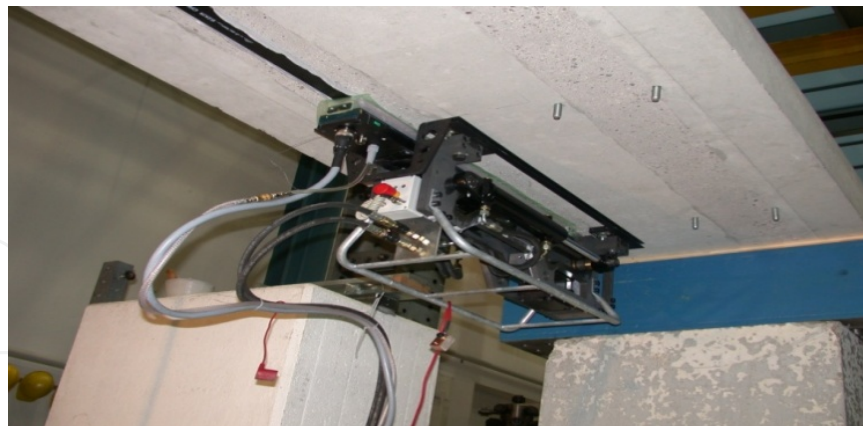
Figure 6. New version of the prestressing device developed by Stoecklin & Meier (Meier [10]).
