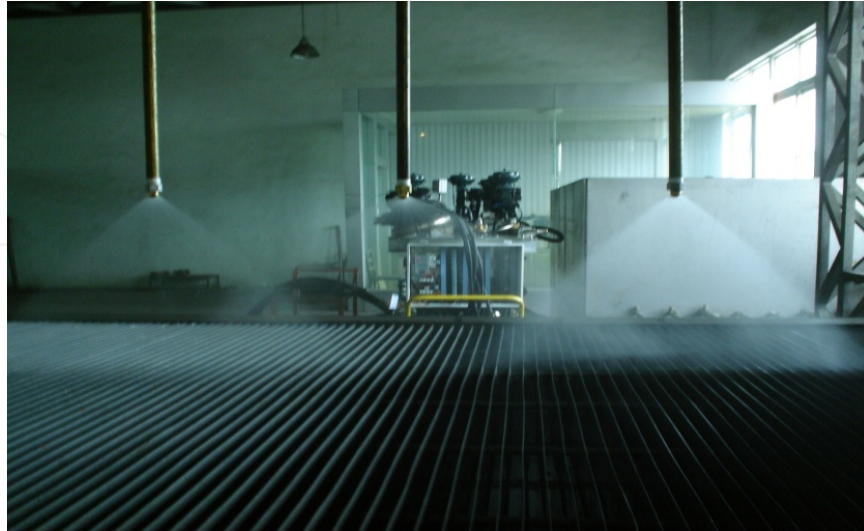
Figure 14. Experimental device of cold characteristics test for cooling nozzles
