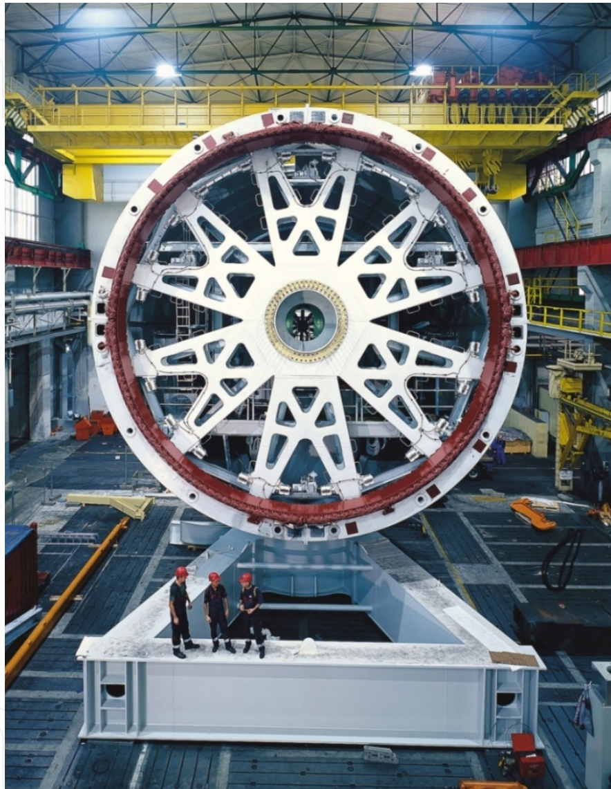
Figure 16. Example of a direct drive MW wind turbine generator.
