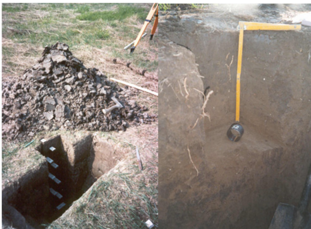
Figure 7. Collection of untouched soil samples
