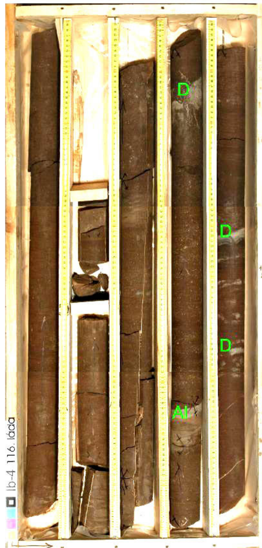
Figure 6. Reddish brown albitic analcite-bearing claystone with interbedded aleurolite (Al) and dolomite (D) layers (Ib-4, 591-596 m).
