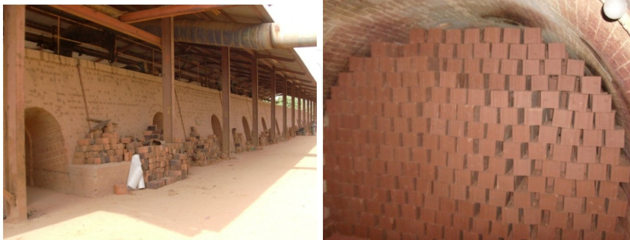
Figure 8. Tunnel kiln and its inner chamber
