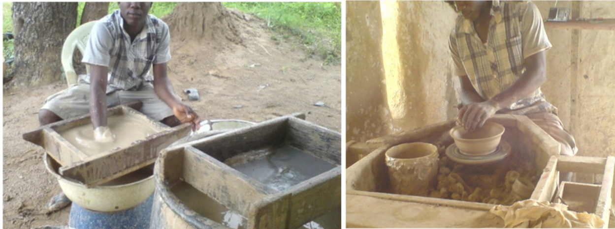
Figure 13. Local clay body preparation and clay throwing process at Maraba Pottery Centre
