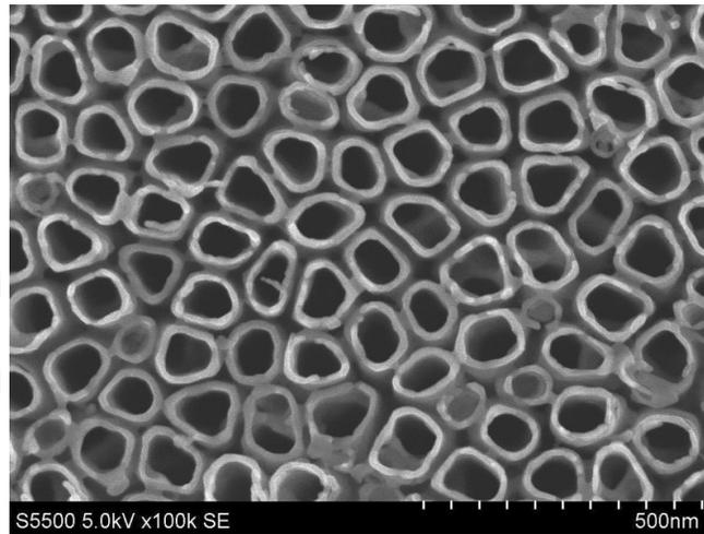
**Figure 8.** SEM image of the TiO<sub>2</sub> nanotubes after annealing in air at 600°C for 2 hours
