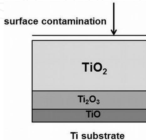
**Figure 3.** Schematic illustration of native oxide layer on Ti.
