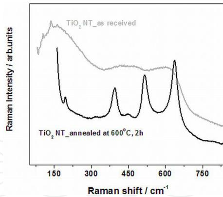
**Figure 11.** Normal Raman spectra of TiO<sub>2</sub> nanotubes: as-received and annealed at 600°C. In as-received state we can observe only a broad spectrum from amorphous TiO<sub>2</sub> structure. At 600°C the NR spectrum shows peaks around 635, 520, 390 cm<sup>-1</sup>, which correspond to anatase phase. Our measurements for annealed TiO<sub>2</sub> nanotubes are in good agreement with data presented in the works [68,69].
