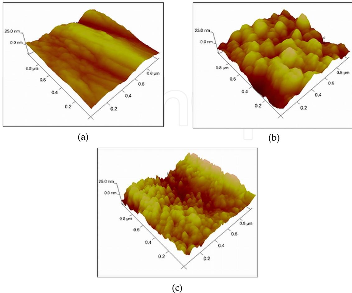
**Figure 7.** AFM images of untreated Ti (a) and chemically treated in NaOH solution (b), H<sub>3</sub>PO<sub>4</sub>+H<sub>2</sub>O<sub>2</sub> solution (c)
