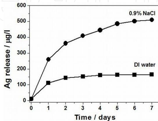
**Figure 27.** Amount of silver released from TiO<sub>2</sub> nanotubes loaded with 0.01 mg/cm<sup>2</sup> of Ag.
