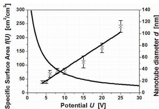
**Figure 12.** The relationship between the diameter of the titania nanotubes and the resulting specific surface area as calculated from the proposed geometric model (more details is given [71]).
