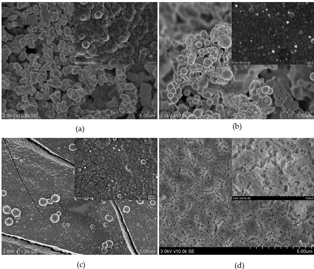
**Figure 13.** SEM images (top view) of Ti after chemical/electrochemical treatment and after subsequent immersion in Hanks' solution – 7 days, temperature 37°C : a – NaOH, b – H<sub>3</sub>PO<sub>4</sub>+H<sub>2</sub>O<sub>2</sub>, c – TiO<sub>2</sub> nanotubes. SEM image of the electrodeposited Ca-P coating on a Ti from Hanks' solution (d).
