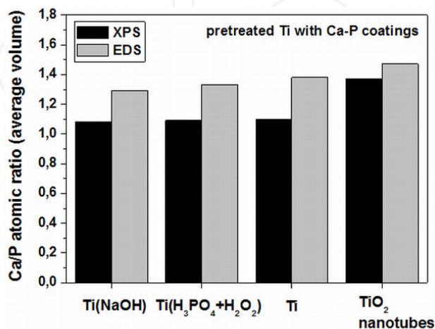
**Figure 17.** Results of the XPS and local EDS analysis (Ca/P atomic ratio) of calcium phosphate coatings electrodeposited on pure Ti or deposited on chemically/electrochemically treated Ti.
