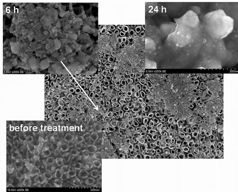
**Figure 25.** SEM image of typical TiO<sub>2</sub> nanotube layer (before treatment) formed at  $V_{\max} = 20$  V and loaded with 0.01 mg Ag/cm<sup>2</sup> and SEM images of TiO<sub>2</sub> NT with the same amount of Ag after immersion in Hanks' solution for 6 h and 24 h.
