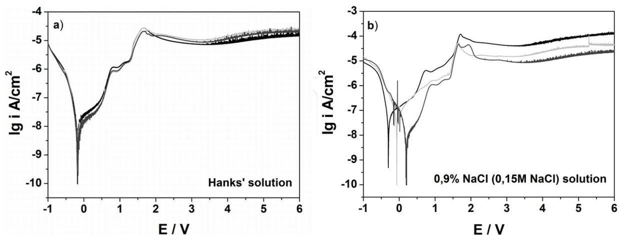
**Figure 4.** Potentiodynamic polarization curves of Ti (initial state) in Hanks' (a) and 0.9% saline solution. The curves were recorded at room temperature (25°C). An AutoLab PGSTAT 302N potentiostat/galvanostat were used in the standard 3-electrode configuration. A normal silver chloride electrode (Ag/AgCl (3M KCl)) and a platinum wire electrode were used as reference and counter electrodes, respectively. A slow potential sweep rate of 1 V/h was applied.
