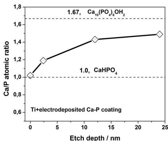
**Figure 18.** Composition of Ca/P concentration ratio vs. sputtering depth for a coating electrodeposited on Ti.
