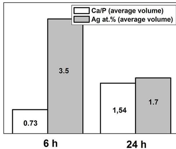
**Figure 26.** Results of EDS analysis Ca/P atomic ratio and silver concentration (average volume) of calcium phosphate coatings deposited on TiO<sub>2</sub> nanotubes loaded with 0.01 mg/cm<sup>2</sup> of Ag after various immersion times in Hanks' solution: 6 h, 24 h.
