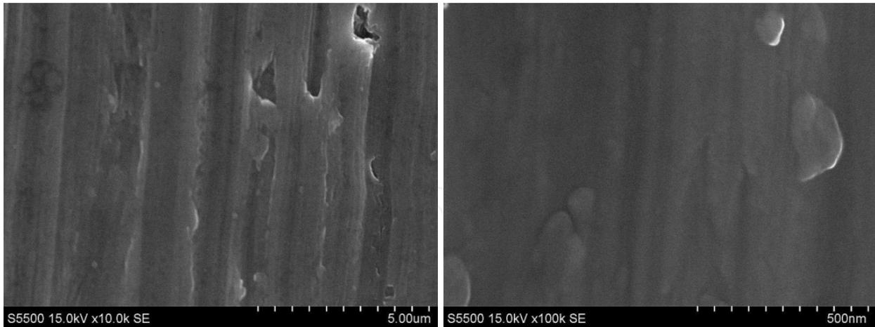
**Figure 1.** Surface morphology of Ti foil (initial state, unmodified Ti).
