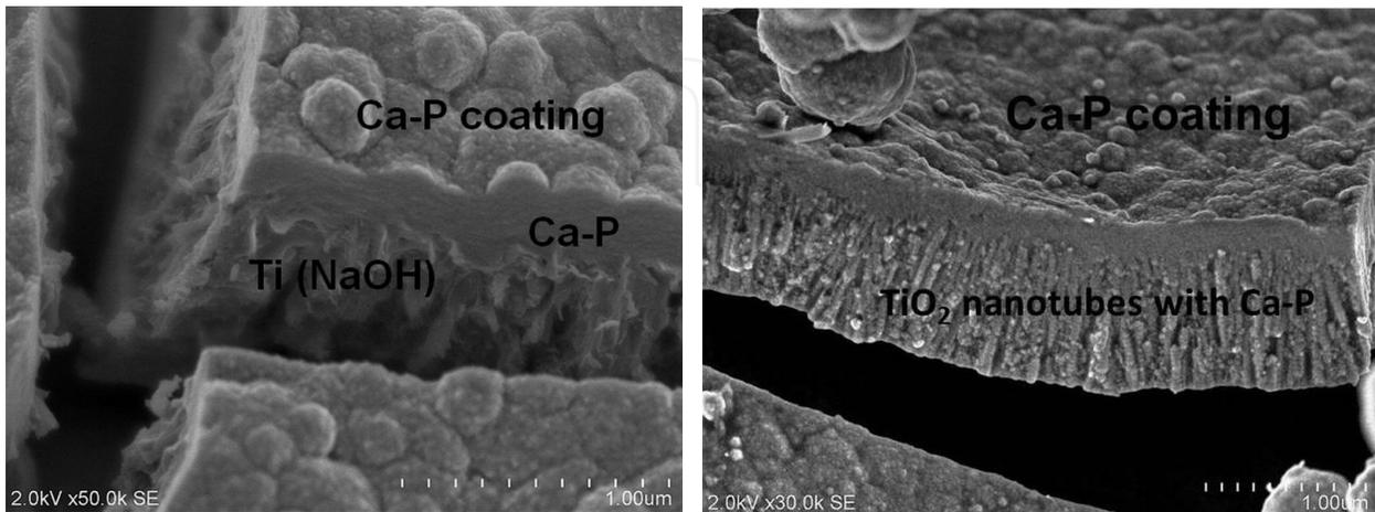
**Figure 14.** SEM images of a cross-section of the titanium oxide porous structure with a deposited calcium phosphate coating.
