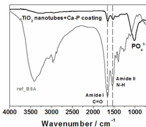
**Figure 20.** FTIR spectrum of TiO<sub>2</sub> nanotubes coated with calcium phosphate (Ca-P) after 7 days' immersion in Hanks' solution. Reference spectrum for pure albumin is also given.
