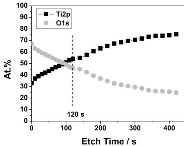
**Figure 2.** Normalized XPS profile for native oxide layer on Ti.
