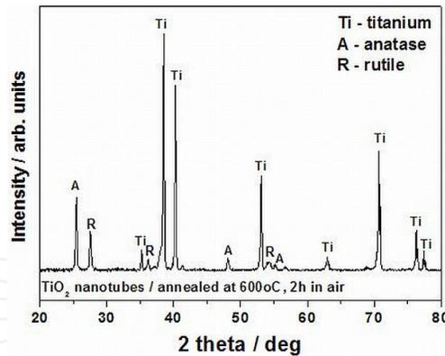
**Figure 10.** XRD spectrum of TiO<sub>2</sub> nanotubes formed on a Ti substrate after heat treatment.
