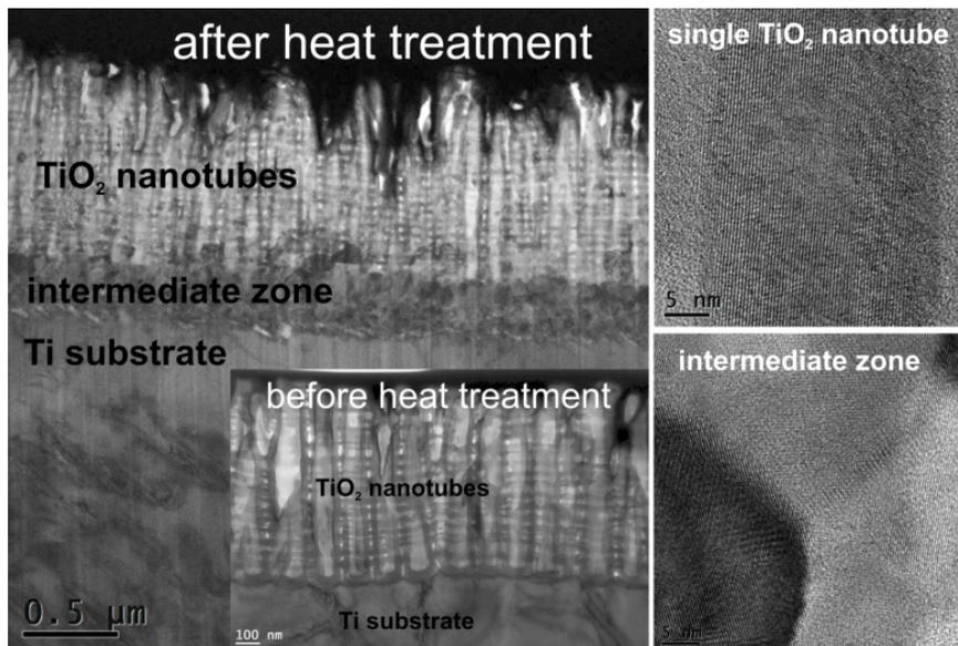
**Figure 9.** TEM image of a cross-section of the porous structure before and after heat treatment in air at 600°C, 2 h. High-resolution STEM images of the intermediate zone (interphase region) and single TiO<sub>2</sub> nanotube.
